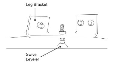
A wrench may be needed to thread the Swivel Levelers into the bottom of the Rail Support Legs.
