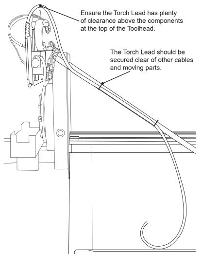
The Customer should ensure the Torch lead is secured so it is clear of the cables at the top of the Toolhead. It is recommended that the Torch lead be secured so it loops up above the components at the top of the Toolhead.
