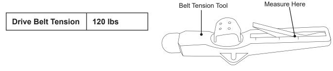
To adjust Drive Belt tension, use a  $\frac{3}{4}$  in. socket and ratchet or  $\frac{3}{4}$  in. wrench to turn the adjustment nut that was installed in section 4.2. Turn the nut clockwise to add more tension.
