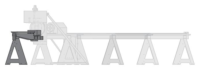
On machines without a Powered Gate the Beak will attach to the Head using eight bolts. If the machine is equipped with a Powered Gate the Beak will attach using four bolts.
