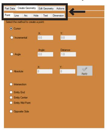
In Edit Flat, Click Create Geometry. An interface will open with tabs where the Operator can choose to create different geometry on the part. After geometry is added to the part, an action will be given to each specific geometry.
