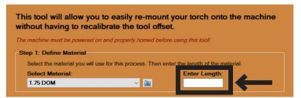
Enter the length of the material that will be loaded into the machine.
