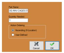
This will open an interface that will allow the Operator to enter or change a Part Name and a Quantity Needed. The Operator can also change the Action Ordering. Click OK. Repeat this process as needed for the parts listed.
