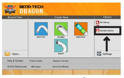
To begin the Torch Mount procedure in Dragon CAM, go to Machine Library. The Machine Library will show any Dragon A400 machines integrated with the computer. This will likely only show one machine. The Operator should choose the machine that will be calibrated in this procedure.
