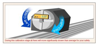
Calibrating the Chuck requires placing a small level or angle finder on the Chuck teeth. Once the level or angle finder is placed, the Operator can jog the Chuck into a level configuration using the left and right mouse buttons. With the Chuck head calibrated to level it is now synchronized with the tool head. This is critical when performing cutting procedures.
