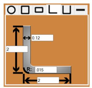
It is advised that the Operator enter .015 as the corner radius in the material dimensions when processing angle material.
