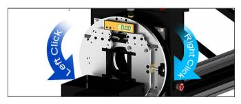
Calibrating the Powered Gate requires the Operator to place a level on the Gate. As indicated on the screen, the best place to do this is by placing the level on the top of the front adjustable Gate as shown in the image on the screen. Use the right and left mouse buttons to jog the Powered Gate into a level position.
