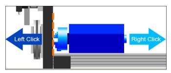
Max travel length is determined by moving the Trolley as far forward as possible. It is recommended that the Operator move the Trolley forward so there is a minimal amount of space visible between the front surface of the Chuck teeth and the Toolhead when viewing from the side of the Toolhead. If there is no space visible the Trolley is too far forward.
