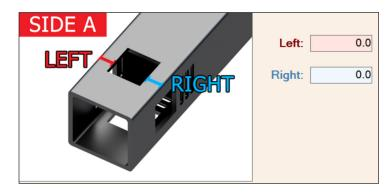
The program will ask the Operator to measure the distance of the left hand and right hand side of the hole to the edge of the material.
