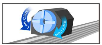
The program will then ask the Operator to verify the Chuck is moving properly in relation to the computer mouse controls.
