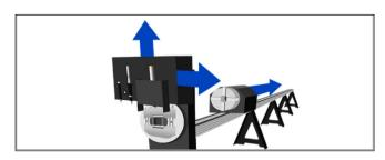
The Operator will be asked to perform the machine's Homing process. Before beginning the homing process the Operator should assure the Gate Lead Screws are in the 12 o'clock and 3 o'clock positions. To begin the Homing process click the image in the interface
