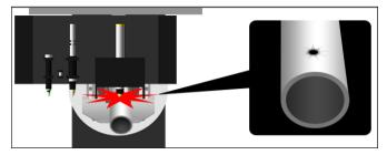
Click the Pierce Hole button to initiate the Torch action. The Torch will move to the material and fire once. Depending on what the machine amperage is set at the Torch may only gouge a hole, it may not pierce through the material. This is sufficient for calibration purposes.
