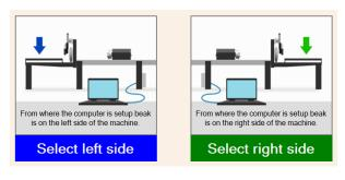
The procedure will then ask the Operator to choose a left side and a right side of the machine based on where the Operator has placed the computer.
