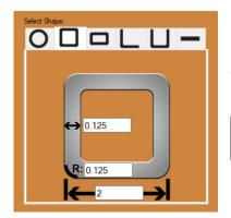
Select the shape of the material that will be used in the Select Shape box on the right hand side of the interface. Enter the dimensions of the material in the appropriate text boxes. Enter a name for the material.
