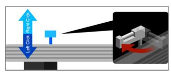
The Lifter Station Switch establishes the the engagement position for the Material Support Lift.
