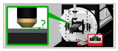
The program will ask the Operator to record the gap distance between the Torch and the material for each side of the material. This can be accomplished using a set of feeler gauges and calipers as outlined in section 1.1.7.
