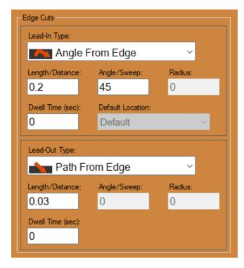
In the Lead In/Out settings, under Edge Cuts, set the Lead-In Type to Angle From Edge, the Length/Distance to **0.2** in. and the Angle/Sweep to 45-degrees.
