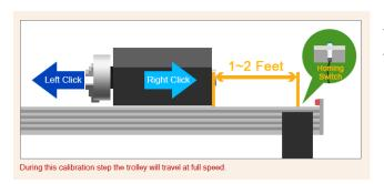
The computer will ask the Operator to use the mouse to jog the Trolley within 1-2 feet of the end of the Rail.
