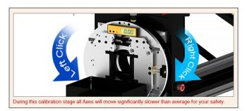
Calibrating the Powered Gate requires the Operator to place a level on the Gate. As indicated on the screen, the best place to do this is by placing the level on the Gate as shown in the image on the screen. Use the right and left mouse buttons to jog the Powered Gate into a level position.
