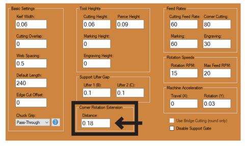
When processing angle and channel material, or any material with a sharp radius, it is necessary to slow the Torch and give it a larger radius as it passes over the corner. Bend-Tech has calculated a formula for this:
