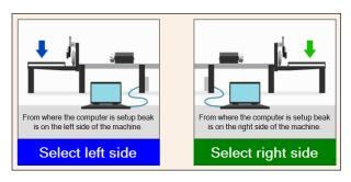
The procedure will then ask the Operator to choose a left side and a right side of the machine based on where the operator has placed the computer. Choose which side the computer is placed.
