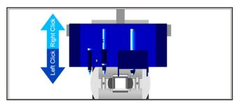
Next the program will ask the Operator to use the computer mouse to verify the Toolhead is moving properly up and down.
