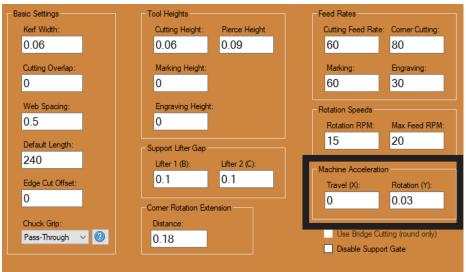
To set Y-Axis acceleration, on the Bend-Tech Dragon home interface, under Library, click Tube Library, then click the Machine icon. In the bottom right, in the Machine Acceleration box, change the Rotation (Y) value to .030 in.
