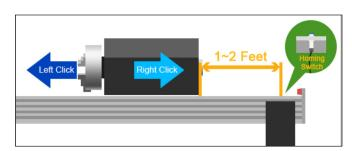
The computer will ask the Operator to use the mouse to jog the Trolley within 1-2 feet of the end of the Rail.
