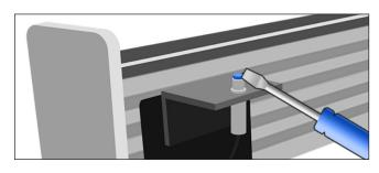
Homing Switch operation is checked by touching the face of each switch with a metal tool, such as the blade of a screwdriver.
