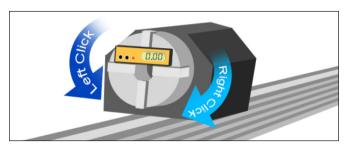
Calibrating the Chuck requires placing a small level or angle finder on the Chuck teeth. Once the level or angle finder is placed, the Operator can jog the Chuck into a level configuration using the left and right mouse buttons. With the Chuck head calibrated to level it is now synchronized with the Toolhead. This is critical when performing cutting procedures.
