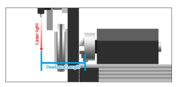
Using a tape measure, and with the Trolley in its maximum travel position on the X Axis from the previous calibration step, feed the tape through the gate to the base of the Chuck. If the Trolley is in the correct position the measurement from the base of the Chuck to the laser should be 13-13.125-inches. This is the machine's Dead Zone.
