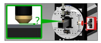
The program will ask the Operator to record the gap distance between the Torch and the material for each side of the material. This can be accomplished using a set of feeler gauges and Vernier calipers. Before beginning, verify the Gate Lead Screws are in the 12 o'clock and 3 o'clock positions.
