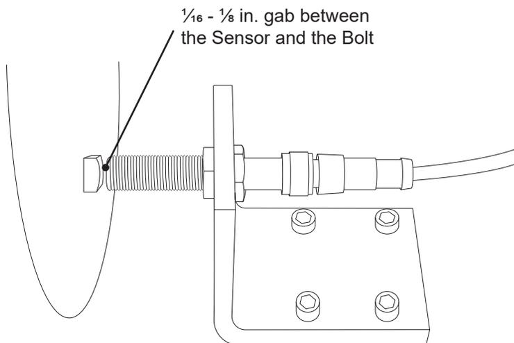
4. If the gap is not within spec, loosen the nuts on the sensor and adjust accordingly.
