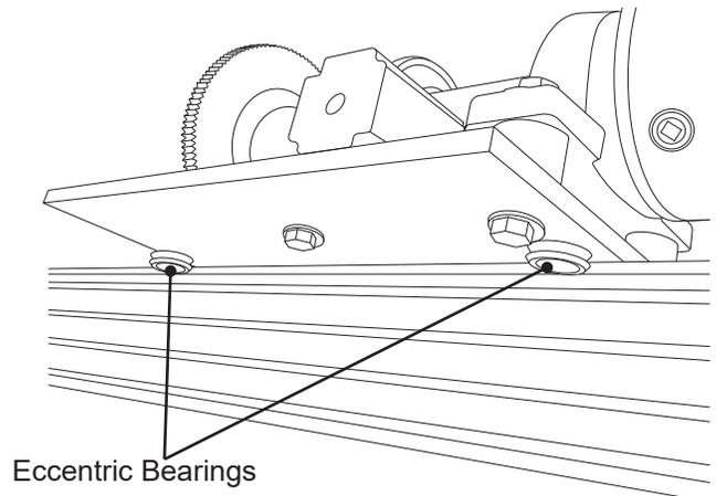
bearing mount nut on the top side of the Trolley. Loosen the bearing mount nut just enough to allow adjustment of the bearing using the flat wrench. Adjust the bearing so the Trolley rides smoothly along the Rail with minimal effort and not side-to-side or up and down play.
