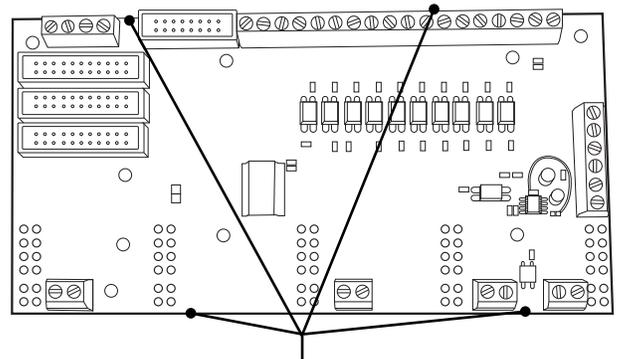
Hold the Breakout Board on the sides and gently pull it off the motor drivers.
