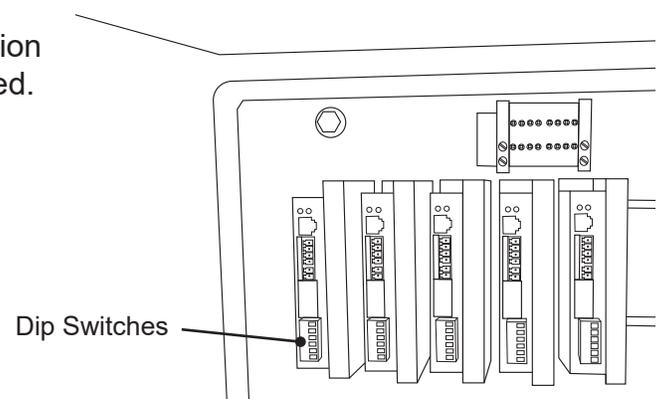
6. Using a  $1\frac{1}{32}$  in. nut driver or small socket and extension, remove the top nut securing the Motor Driver. Loosen, but do not remove, the bottom nut. Lift the Motor Driver slightly upward and tilt the top out to remove.
