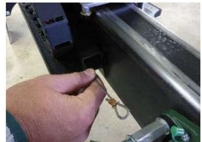
Next, attach the loop on the end of the cord to the bolt on the very rear end of the chuck trolley.
