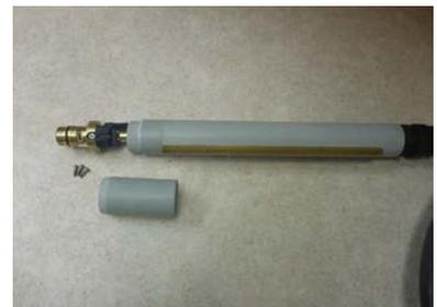
**Step 4:** Finally, loosen the next ceramic section all the way and maneuver it to one side in order to slide the brass teeth out from its slot on the torch.
