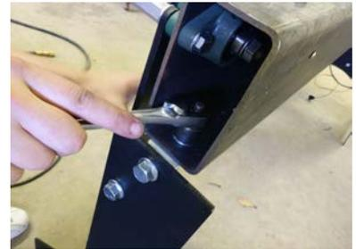
**NOTE:** The supports used to prop up the bulk of the new rail (Not Included) should raise the bottom edge up roughly 29 - 29 1/4 inches off the ground to match the height of the stock rail.
