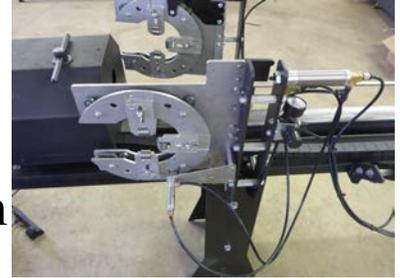
**Step 1: For Round** – Position the center gate in line with the bolt holes in the center location of the rail. **Tip:** The lip underneath the rail may prevent you from butting the gate up to the rail entirely, so you may have to lift up on the rear of the machine to be able to slide the gate into position.
