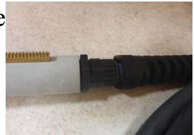
**Step 3:** Then, loosen the section of the ceramic torch nearest the head, remove it and set it aside. **Note: The bulk of the torch will turn; not the section nearest the head.**
