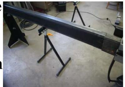
**Step 2:** Line up the bare end of the new rail with the 3 foot stock rail in preparation to transfer the chuck to the new rail.
