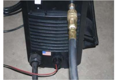
**Step 9:** Attach your air hose to both the back of the torch power source and to the back of the machine located on the electronics guard plate.
