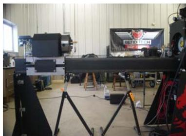
**Step 4:** Working on the front of the machine now, take the beak and attach it to the front face using the **ratchet** and **3/4 inch bolts** provided.
