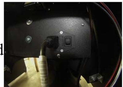
**Step 7:** Attach the alligator clamp from your torch power source to the ground wire underneath the machine's electronics core.
