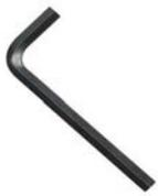
**Step 4:** If you have loosened the bottom plate on the chuck as mentioned in the previous tip, use the **5/16 inch hex wrench** to tighten the bottom bolts now.
