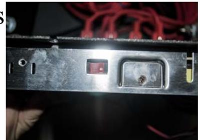
**Step 4:** Return the electronics core to its original position and secure the panel with the four screws using the **phillips head screwdriver**. Then, make sure to secure the electronics guard plate with the four **3/8 nuts**.
