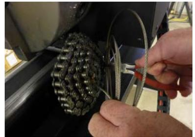
**Step 7:** Guide the end of the chain and steel cord through the chain guide block and around the machine's sprocket. Pull it tight to allow the teeth of the sprocket to settle within the links of the chain.
