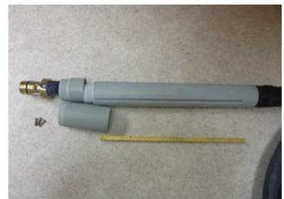
**Step 5:** Reassemble the torch in the order it was taken apart (minus the brass teeth), and make sure to line up the pin inside of the torch with the first ceramic section that was removed.
