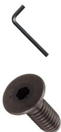
**Step 11:** The track with the connector wires inside of it should rest on top of the square tube. Using the **1/8 inch hex wrench**, screw in the **two fastener screws** into the pilot holes where the track meets the cable wrap. This is located on the rail nearest the back leg.
