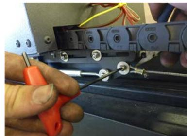
**Step 10:** The **turnbuckle** and the **two hex bolts** above it on the support plate will adjust so that it doesn't rest on the square tube below it by tightening up the slack on the chain and cable.
