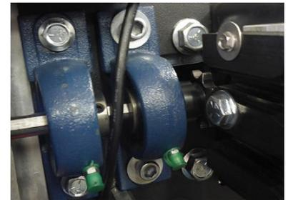
**Step 2:** Align the center of the guide block with the inner chain gear then tighten the 2 bolts of the block.
