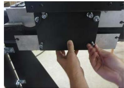
**Step 2:** As a recommendation, we urge you to degrease the rail and wipe it down with a rag to remove any unnecessary shipping grease before sliding the chuck on. This will make the transfer process easier and keep your machine running as smooth as possible.
