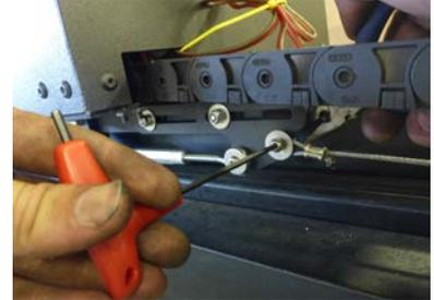
**Step 10:** The **turnbuckle** and the **two hex bolts** above it on the support plate will adjust so that it doesn't rest on the square tube below it by tightening up the slack on the chain and cable.
