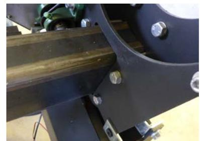
There should be a small gap between the chain guide block (from the previous step) and the sprocket in front of it (attached to the machine head).
