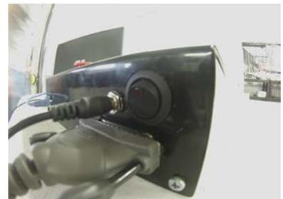
**Step 11:** Flip the switch on the electronics core panel. The machine motors will turn on and begin humming to indicate that the machine is running.
