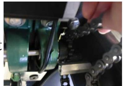
**Step 8:** Lead the cord (on the end of the chain) through the one inch square tube located along the side of the rail. Then, guide the end of the cord under the first bolt and around the pulley so that it rests in the groove on the top edge of the pulley.
