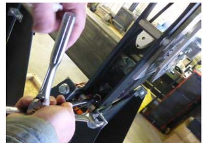
the rail as you remove the bolts. Be sure to support the stock rail as it will become loose.
