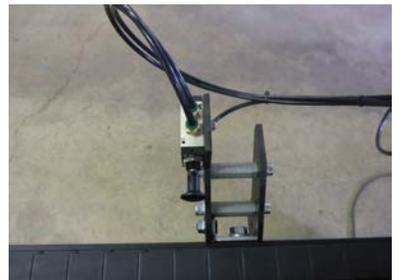
**Step 4:** Push the air line into the bottom of the air pressure regulator to connect it.
