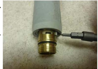
**Step 6:** Tighten up all of the parts by screwing on the rear clasp last, then return the **3 phillips head screws** to their original positions at the head of the torch.
