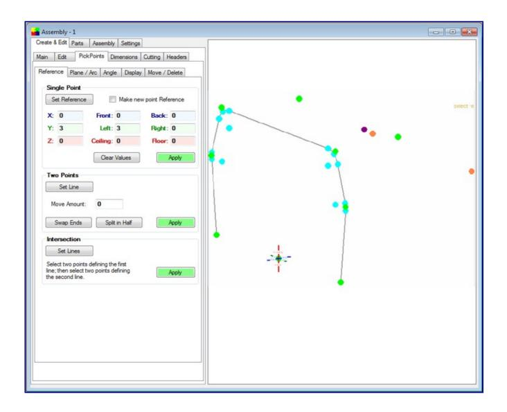
Step 4) Working off of the newest PickPoints (the points in the picture as dark blue) I went back to using the "Angle" method and placed and angle down of 80 degrees and a short distance. In this case the distance doesn't matter because I am just trying to create a line of direction.
