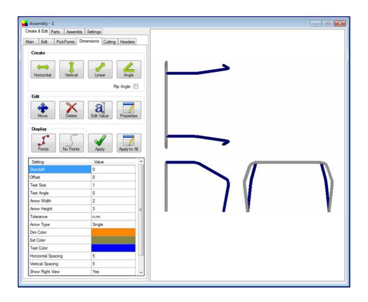
Step 8) Use the "Parts" tab and select the part from the list. Use the "Send to XYZ" command button to send it and find your cut length, bend locations, angles and rotations.
