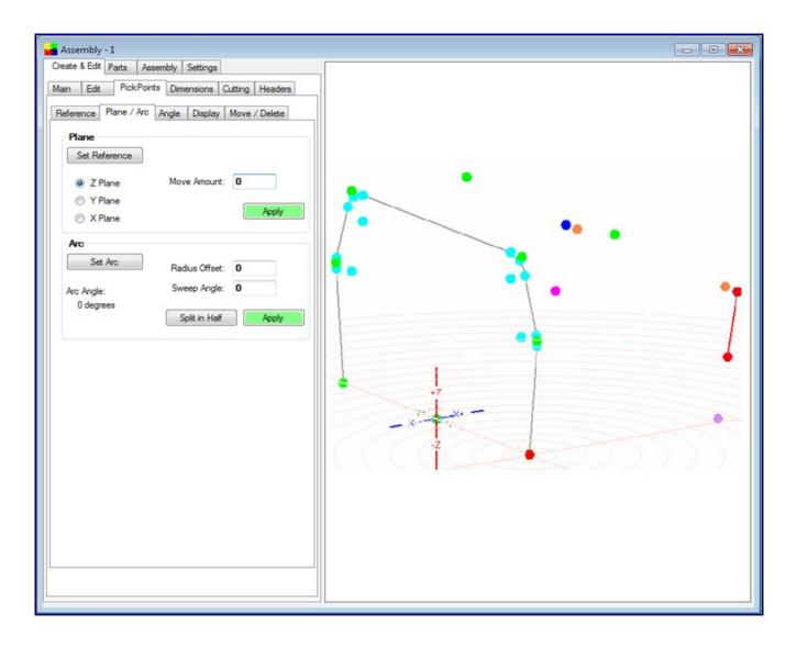
Step 6) I am going to assume for this illustration that the last 2 points we created are at the correct front/back location and at the correct ceiling/floor height, however, the are not at the correct left/right width. In my case I want to make them the same width as the 1st pillar. [again if the width is smaller or bigger, create PickPoints off of the 1st pillar left or right to locate the plane correctly.
