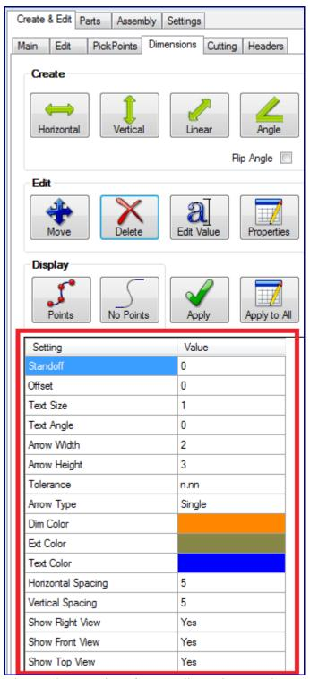
Change these settings for new dimensions or change the settings and select the "Change Dim Setting" for a single dimension that is displayed or "Change All Settings" for all of the dimensions displayed.
