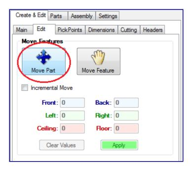
Step 2) **Select ANY PickPoint on the part you are going to adjust.** We are only doing one thing with this step and that is to select the part. Select the easiest point to select the part.
