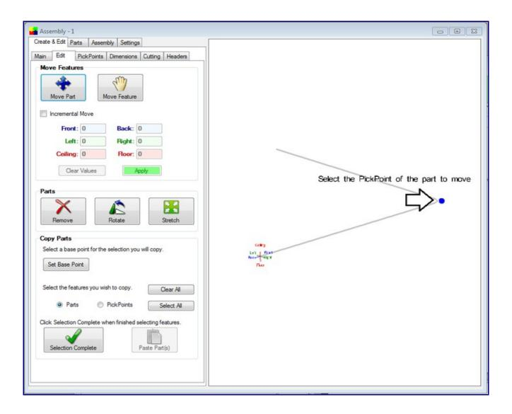
Step 3) **Select the PickPoint on the part that will be the coupler location.** This will be the point of the part that is anchored to the cursor while it's being moved.
