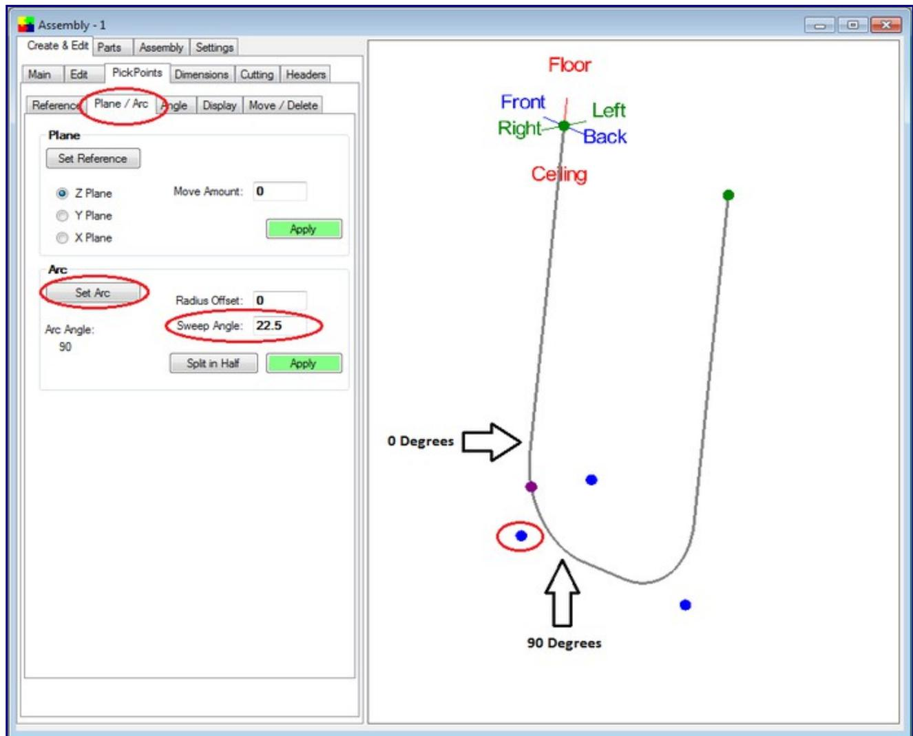
**Note:** The numbers of degrees for the entire arc is displayed above the "Sweep Angle". 0 (zero) degrees is on the arc end which is the start end. The start end was determined by the direction of the part creation.
