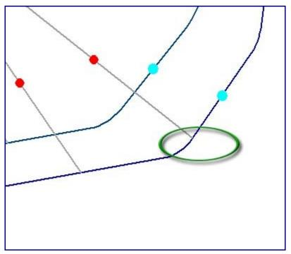
Both the straight tube section and the bend tube section must be selected as our cutting bisectors.
