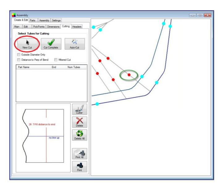
Step 4) Select the dot(s) representing the tube section(s) that our part is going to be cut to. This includes both the straight section and the bend creating the tangent point. You will find the intersecting tubes will turn red. Step 5) Select the "Cut Complete" command button.
