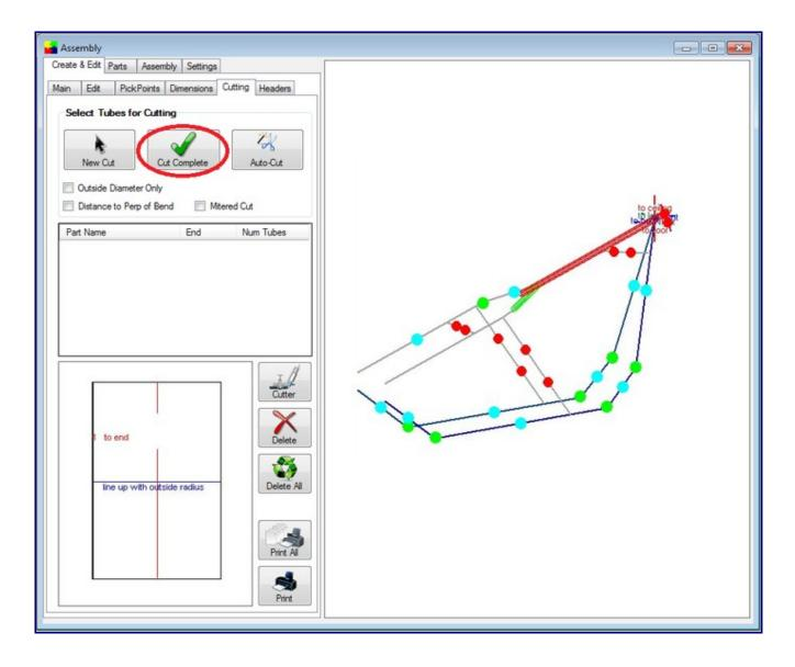
Notice the intersection now has a black and a blue cut marks showing the inside and outside of the material where each meets the intersection part(s).
