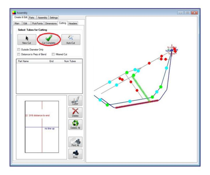
Notice the intersection now has a black and a blue cut marks showing the inside and outside of the material where each meets the intersection part(s).
