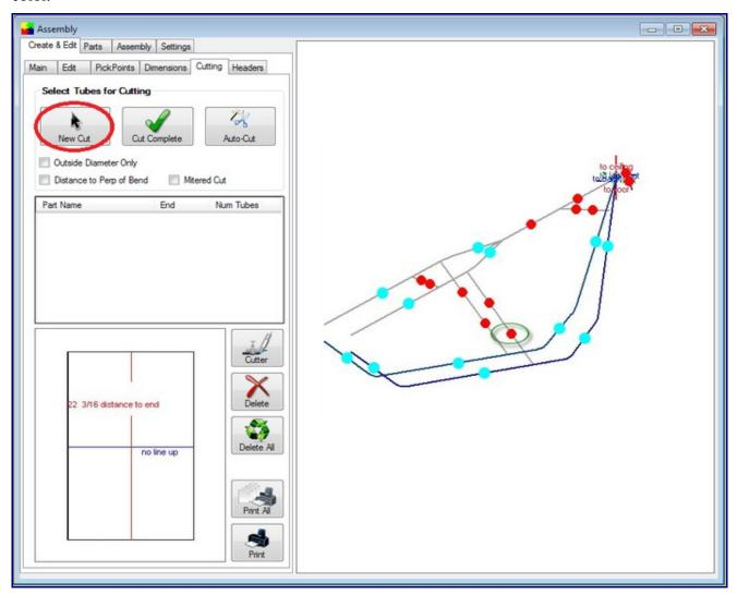
Step 4) Select the dot(s) representing the tube section(s) that our part is going to be cut to. You will find the intersecting tubes will turn red.
