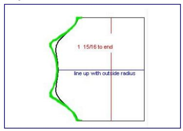
The green cut line represents the cut for a hole say and the black cut line represents that for plasma or grinder line.
