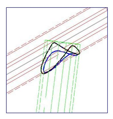
Using a hole saw requires the checking of the outside of the material only. "Check" the option "Outside Diameter Only".
