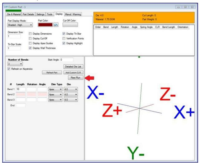
You will see the Rise and Run inputs and underneath those you will see your length and angle will be calculated out to you based on the values of your inputs. You can check the over 90 Degree Bend box and it will bump up your angle to be over 90 degrees but still is calculated out to have the correct Rise & Run. Hit the Use Value button from inside the Rise/Run feature and your lengths and angles will be added to your Custom Part.
