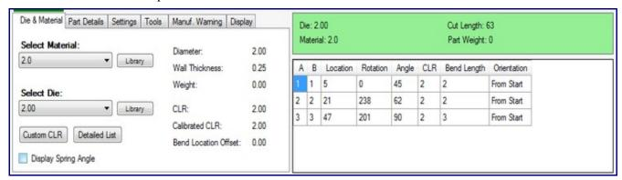
For those that have SE and the Spring Charts filled out you can select the "Display Spring Angle" check box and find the Spring Angles also in the chart.
