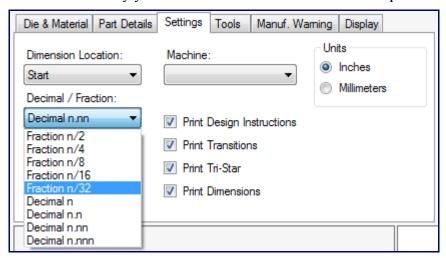
Make sure to change values in the Options menu which can be accessed by clicking the "Tools" menu and selecting "Options". The Decimal/Fraction adjustment menu can be found in the "General" tab, in the Tolerance section under "Lengths".
