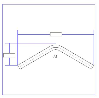
See how the extention line at the top of the peak is representing how the 2 outside edges intersect each other or the "apex".
