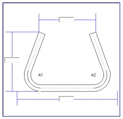
Notice how the horizontal dimension on the bottom of the drawing has its extention lines out to the left and right. This lines are not representing the edge of the material, but the location where the "apex" of the bend is.
