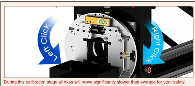
Calibrating the Powered Gate requires the user to place a level on the Gate. As indicated on the screen, the best place to do this is by placing the level on the Gate as shown in the image on the screen. Use the right and left mouse buttons to jog the Powered Gate into a level position.
