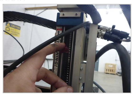
7. Replace the metal sheet covering and push down on the clamp block while you tighten down the screws as shown here.
