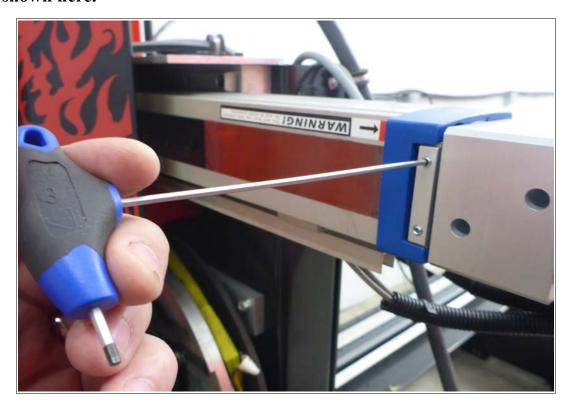
2. Peel back the metal sheet cover to reveal the ball screw inside.
