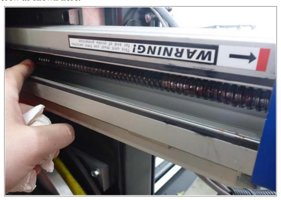
4. Replace the metal sheet covering and using a flat head screwdriver, pry the block as far left as you can while you tighten the screws back down. Make sure that they do catch the covering and clamp down on it properly.
