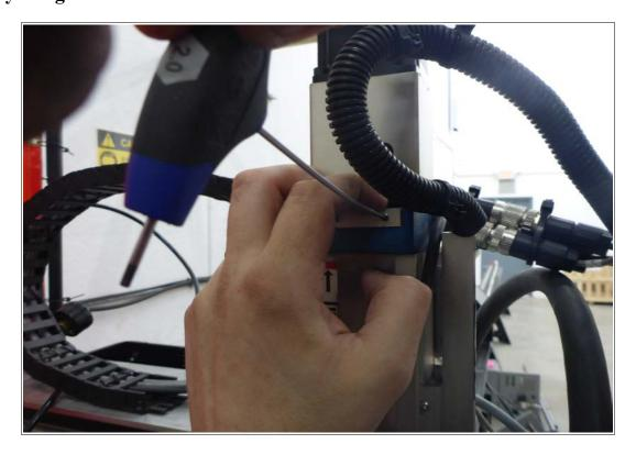
Afterward, we encourage you to jog both axis back and forth, and up and down so that the grease spreads evenly along the ball screws.
