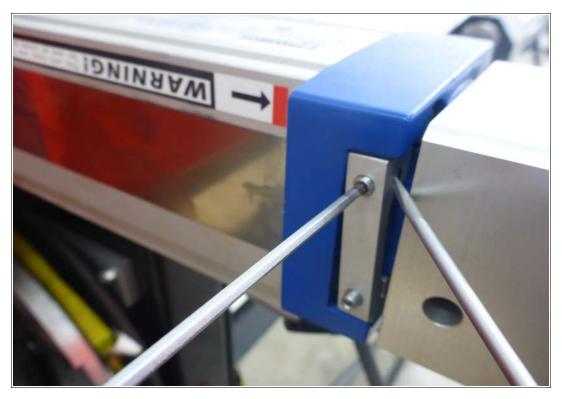
5. Next, locate the A-axis screws here and use a 2mm allen head wrench to loosen them enough to peel back the metal sheet cover.
