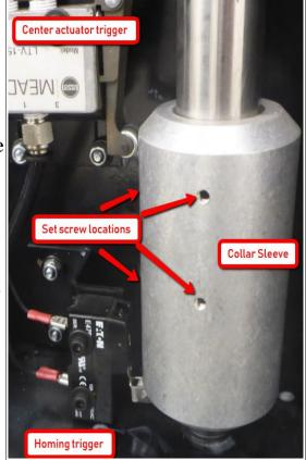
3. At your computer, open the Machine Control screen in the Dragon CAM software, then click on the Home button for the lifter station (the house icon for the B-axis to the far right) so that the collar sleeve lowers to touch the limit switch and then raises off of it.
