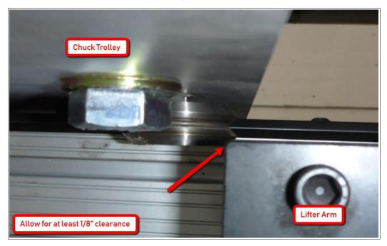
6. Once the collar sleeve has been mounted in its new position, home the lifter once more by clicking the B-axis home icon on your computer and slowly jog the X-axis close to the lifter station once again to ensure that the chuck trolley will clear the lifter arm.
