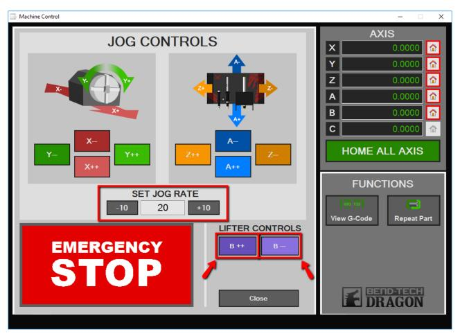
5. If the arm continues to hang up on the rail, repeat steps 3 and 4 until the speed of the lifter arm is quick enough to avoid making contact with the rail and does not activate a limit sensor accidentally.
