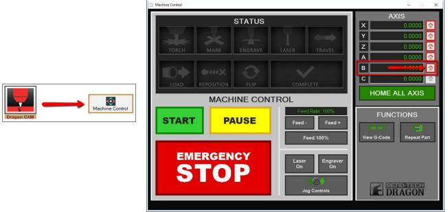
4. Once the lifter is home, click on the Jog Controls in the Machine Control screen and use the X-- and X++ buttons to jog the chuck trolley close to the lifter arm to better judge the distance (if any) needed to lift the collar sleeve.
