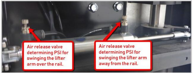
3. Turning the dial COUTER-CLOCKWISE on the RIGHT-MOST air valve will increase the airflow for swinging the arm away from the rail. We advise small adjustments of about a quarter turn and then administering a test.
