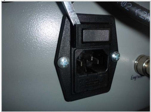
5. With the old switch removed from the control box, insert the new switch into the slot in the same manner as the old switch.
