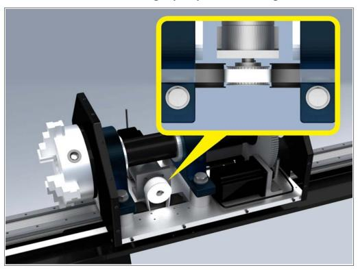
13. With the belt routed as it should be, tighten down the rear clamp block to its original distance from the rear plate.
