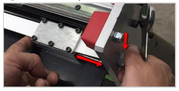
14.Re-attach the chuck housing\* to the chuck trolley with the 26 allen head screws removed earlier.
